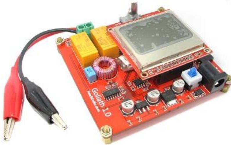
Goliath V1.0 is an opensource simple inductor/capacitor meter. It's based on Arduino, providing a large measure range of inductor and capacitor.
